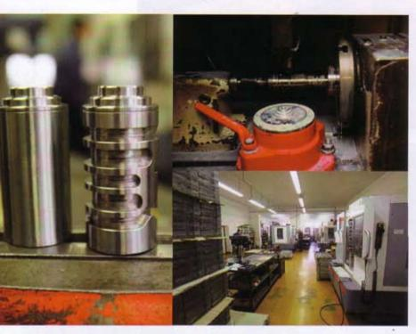
A steel cylinder becomes a desmodromicshaft for gears of 125 B/02KZ engines. Turning and milling are fundamental operations for making grooves in which the gear forks run.
