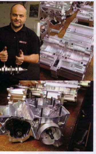
Below, driving shaft with crank at 180° which requires the use of a counter shaft so as to eliminate angular momentum of first order inertial force momentum using eccentric masses to oppose piston phase and turn at the same speed as the driving shaft (aears have the same number of We were told that in
