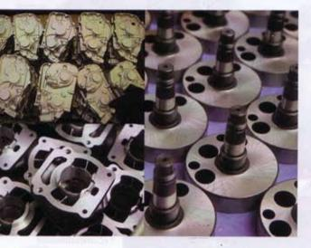
Some of the parts for the latest aearclass 125cc (KZ). Unrefined casing waiting to be machined, cylinders and semi shafts.
